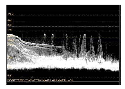
When content is encoded with an Electro-Optical Transfer Function (EOTF) of PQ (ST 2084) or HLG, the waveform display has the additional menu options to show the HDR encoded data converted into "Light Levels".
