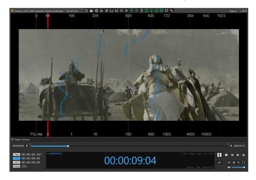
When the content has high random highlights, the traces may appear scattered and difficult to see. Turning the "Filter Line Range" on in the HDR options page will perform a low pass filter on the data to provide a smoother and more visible trace.
