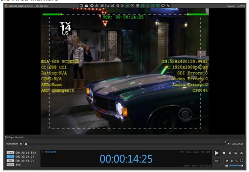
Shows the 4:3 aspect ratio markers in 16:9 content and a safe area marker around the picture. The size of the safe area marker is adjustable in the Options dialog box.
