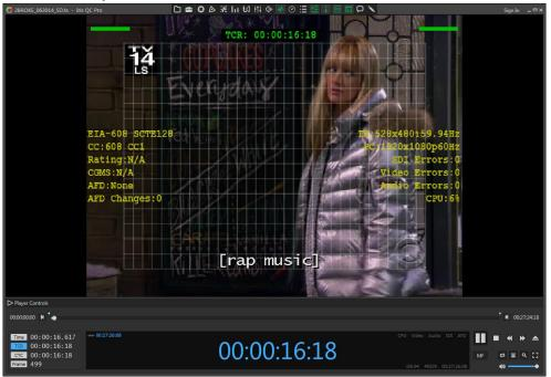
This shows the CEA608 grid of 15x32 or CEA708 grid of 15x42 depending on the caption format selected. This allows verification of text positions within the grid.
