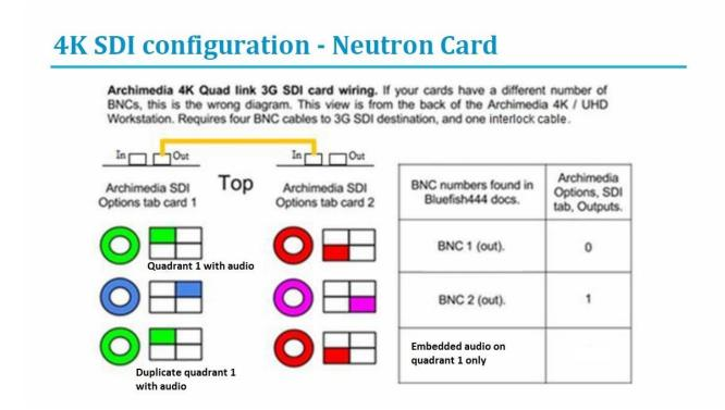
The following picture shows interlock cabling for dual Neutron cards.
