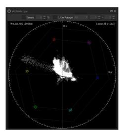
When the "Errors" checkbox is enabled, pixels that are outside of the 100% boundary markers are shown in yellow. The limit can be adjusted within the range of -25% to +25%. A positive value is percentage higher than 100%, a negative value is percentage below 100%. Errors are also logged to the "Timeline" window.
