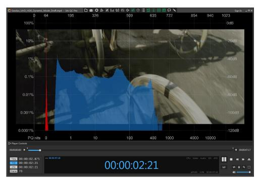
The graticules along the top X-axis indicate the absolute digital level from 0 to the maximum range. The bottom X-axis indicate the same level in nits for PQ or percentage of light level for HLG. The left Y-axis indicate the percentage of values within the frame and the right Y-axis indicate that percentage in decibels (100% = 0 dB).
