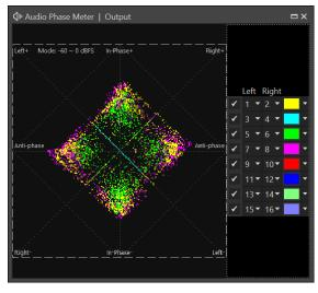
The audio phase meter shows the phase relationship between any two audio channels. There are 8 traces available for view. Each trace can select between any two channel between 1 and 16. When the two channels are in phase, the trace appears vertically (y-axis). When the two channels are out of phase (anti-phase) the trace appears horizontally (x-axis). Predominantly left or right channels appear in the diagonals (45 degree) positions.
