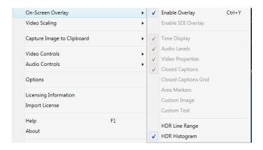
This option only applies if the content is HDR. The HDR Histogram shows the distribution of levels of the video content across the entire frame. For brightness levels that falls below a minimum threshold or exceeds a maximum threshold, that part of the histogram is shown in a different color (the default being red). These limits are taken automatically from the Mastering Display Luminance minimum and maximum metadata values if present.
