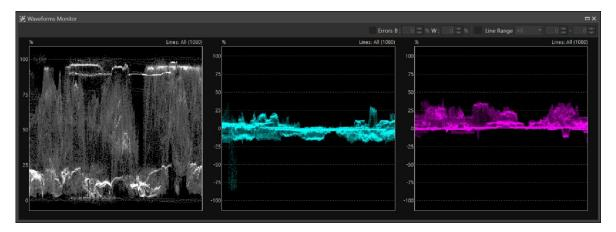
The waveform monitor provides a convenient way to visualize the video across the width of the screen with each line overlaid on top of each other over the time period of one frame. The markers of 0%, 75% and 100% represent the video levels according to the source file resolution and its video standard. YCbCr formats are displayed as Y – Luminance (white), Cb – Blue-Green (cyan) and Cr – Red-Green (magenta). RGB formats are displayed as Red, Green and Blue.
