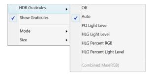
For PQ, the light level is defined as nits (cm/d2) and for HLG, it is defined as percentage of light level. The waveform can display the combined maximum of all three RGB components or as separate RGB waveforms.
