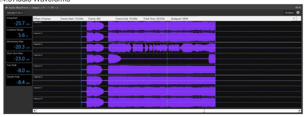
The Audio Waveforms window shows the analog waveform across the channels at the same time position. The center position of the green dotted line represents the top of the current frame, and the yellow dotted line represents the end of the current frame. The distance between the green and yellow markers represents the period of 1 frame. The scale can be zoomed in and out by the use of the + and – buttons on the top right corner of the window.
