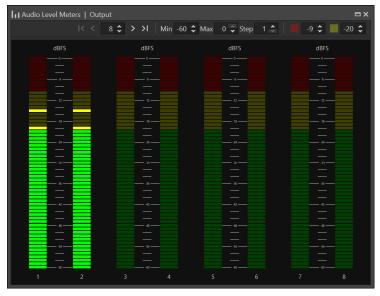
Each meter represents the audio levels of the corresponding output channel. The scale is calibrated relative to 0dBFS (full scale). A context menu on the window has the option to display 'peak hold' at its maximum detected level.
